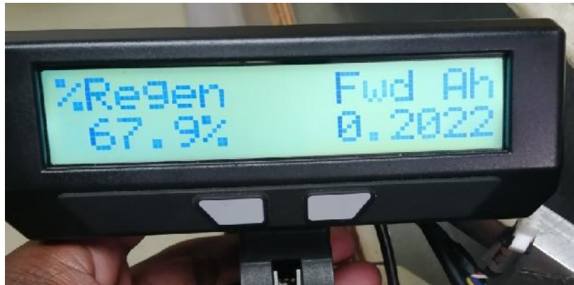
Figure 4: CA Screen Showing Regenerative Braking.
